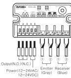
► Connection method for sensor
